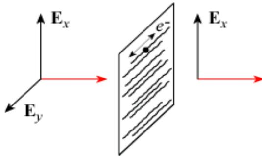
When the electric field of a light wave encounters the polarizer, the component parallel to the direction along which charge flows freely ( $E_y$  in the example) causes the charges to oscillate, thereby absorbing energy and preventing that component from being transmitted. Since charges can not respond to the orthogonal component, that component is passed
