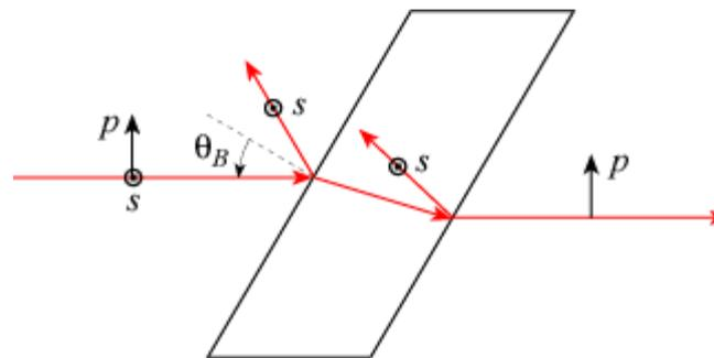
The  $p$ -polarized light is completely transmitted through the window
