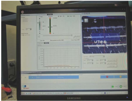
Figure 8 - Scanner GUI & Conoscopic signal on the measured sample
