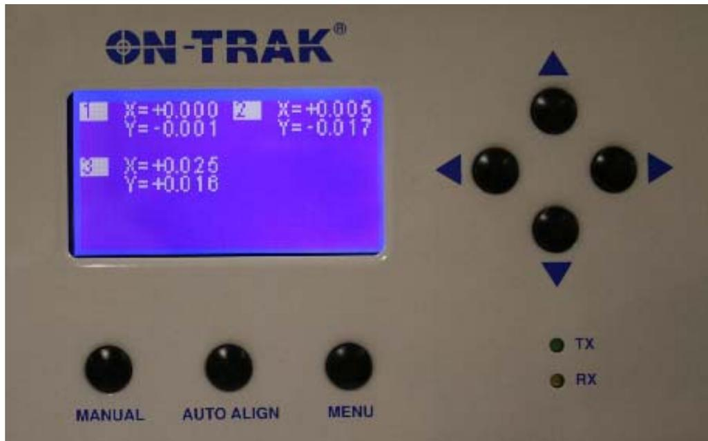
The display will give data for six targets at a time. If additional targets are in the chain, use the down arrow key to scroll down.
