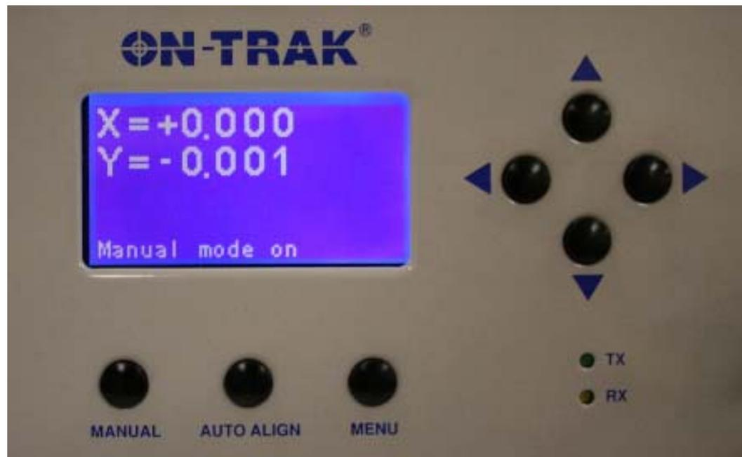
**IMPORTANT – IF THE BEAM PATH TO THE REFERENCE TARGET IS INTERRUPTED DURING AUTOALIGN INITIALIZATION, THE SYSTEM WILL REVERT TO THE MANUAL ALIGN MODE.**
