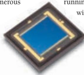
Silicon Position Sensing Detector.
